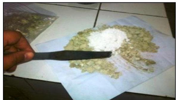
Photo 30: Mixing of clinker with Gypsum
