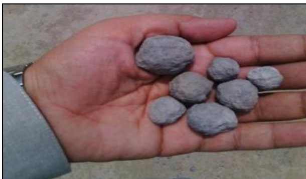
Photo 29: Clinker formed after cooling
