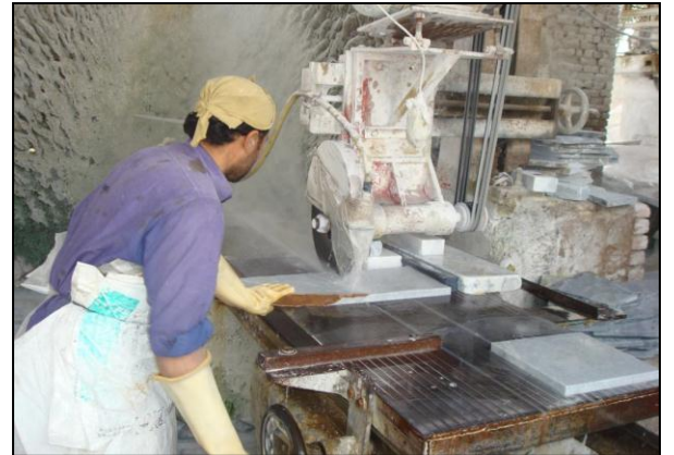
Photo 8: cutting of Slabs into desire size tiles
