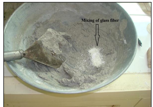
Photo 36: Mixing of raw materials
