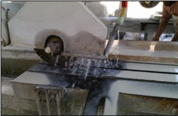
Photo 13: Cooling water usages
