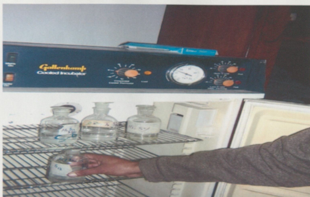
Picture taken while putting BOD bottles in Incubator at 20 °C
