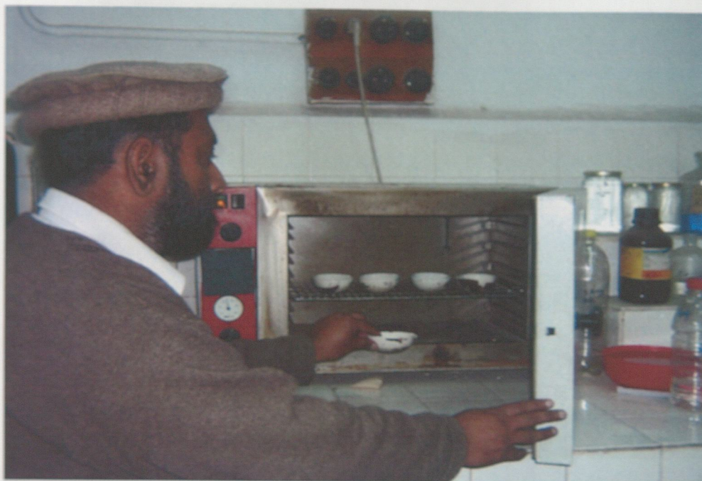
Putting samples in oven for analysis of TDS in lab
