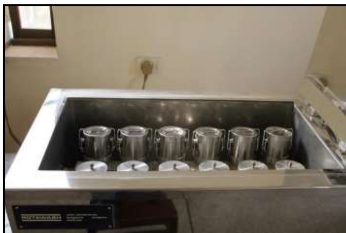
Figure 2.3: Launder-o-meter for Wash Fastness
