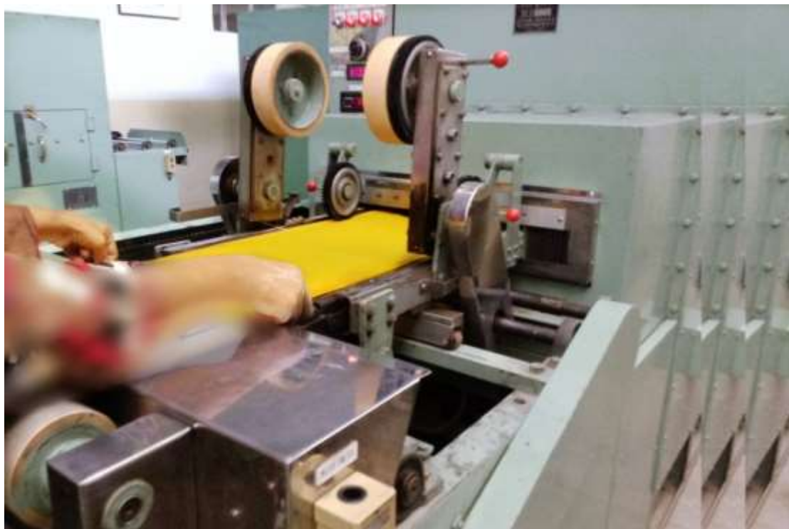
Figure 2.3(a) Front view of Tenter frame (feeding fabric for drying).
