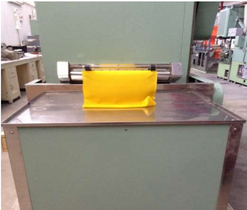
Figure 2.3(b): Back view of Tenter frame (fabric received after drying).
