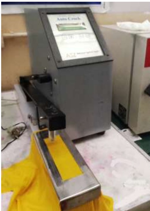
Figure 2.5: Electronic crockmeter/ rubbing fastness tester at work.
